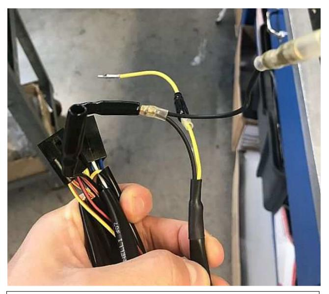
To power the fan connect the black wire of the light wiring with the fan black wire, and then connect the other end of the black wire of the fan wiring to the pin that was inserted in the light wiring
