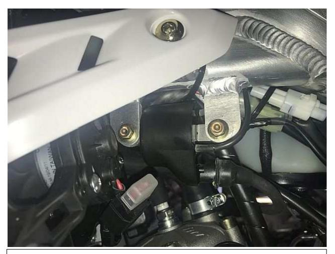
It is recommended to rotate the coil towards the rear of the motorcycle
