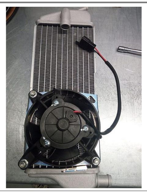
Put the fan on the rear part of the radiator, taking care to keep it as low as possible. It is recommended to fix the fan support with rivets; please be careful when drilling holes in the radiator trying to get down with the drill only a few millimeters, to not damage the radiator.
